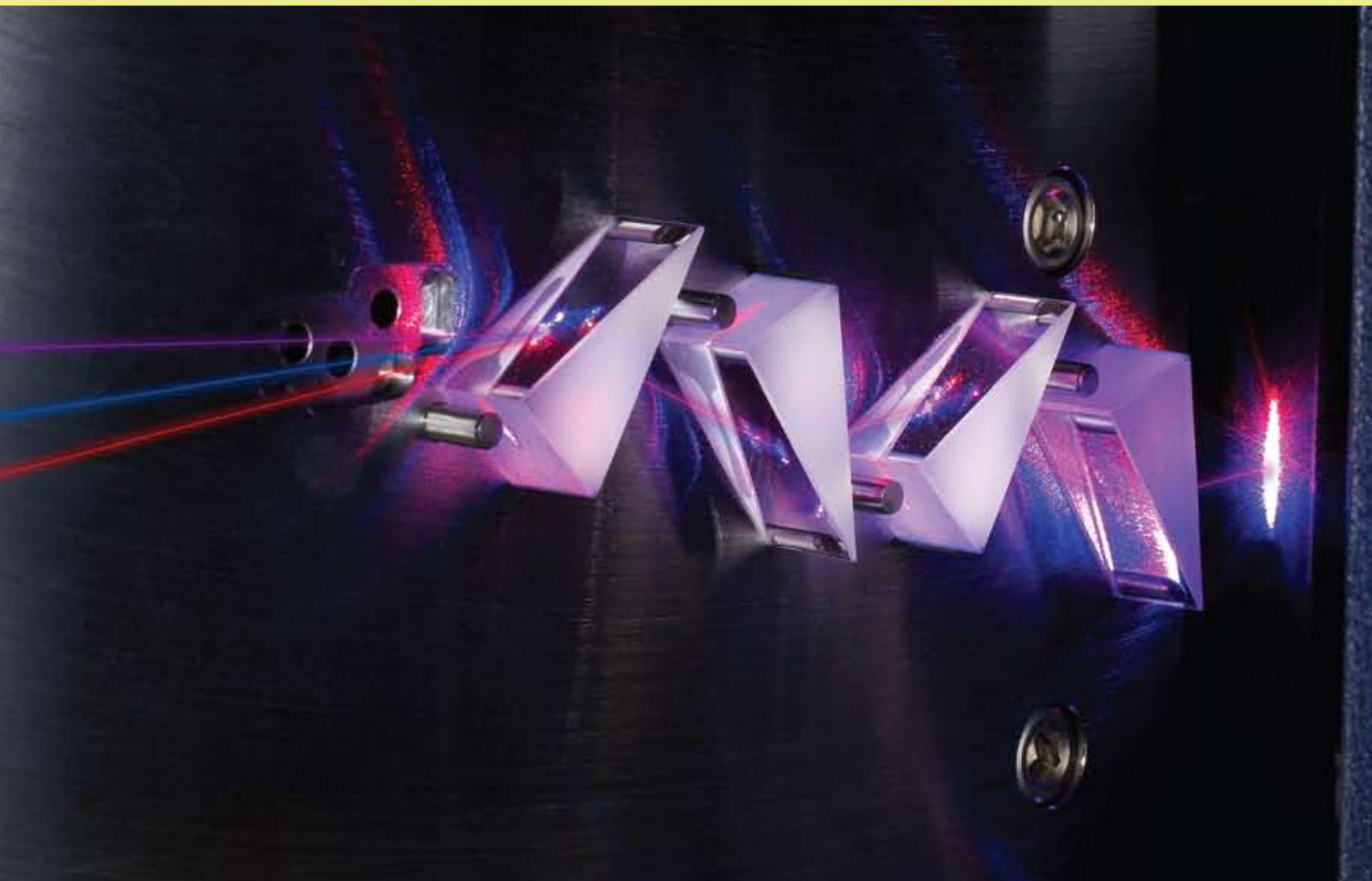
Excitation optics focus the 488-nm, 633-nm, and 405-nm laser beams
